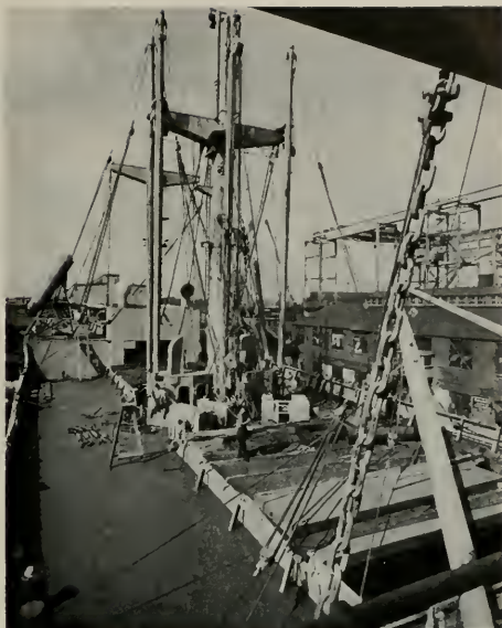
Cargo gear on present C-3 type. Simplified gear on proposed vessel is shown on other cuts herewith.
